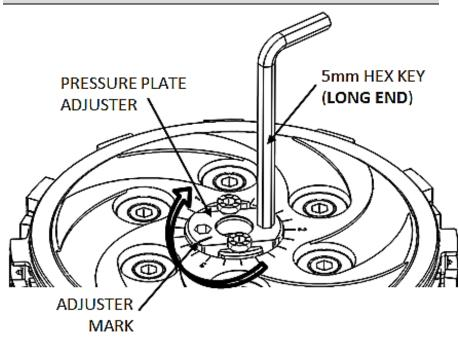
**14.** At this point, make a note of where the tick mark on the Adjuster aligns with the tick marks on the Pressure Plate. This is what's called the **STARTING POINT.**
