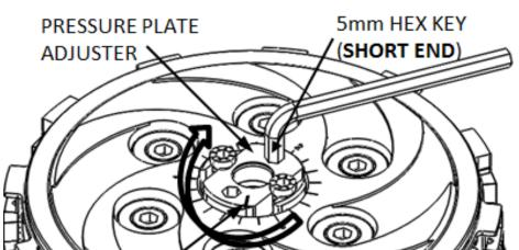
**17.** Once the installed gap is set, use a 4-mm hex key to tighten the two locking Set Screws in the pressure plate adjuster to lock it into place. Tighten the screws evenly in 3-4 steps to 40in-lb. The tops of the set screws should be flush or slightly below flush with the top of the adjuster when torqued correctly. It is **not** necessary to put thread locking compound onto the set screws.
