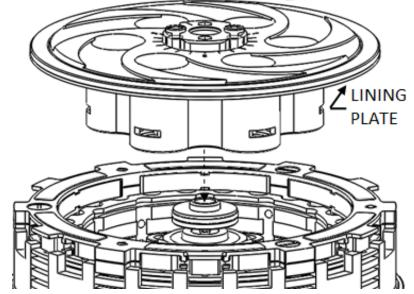
12. Install the pressure plate springs.
