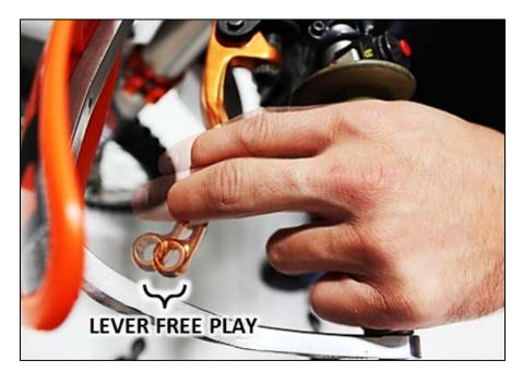
"Freeplay Gain" is the increase of lever freeplay as the auto-clutch engages. This happens when the idle through RPM increase from RPM 5,000 either around with configuration. Freeplay Gain is caused by the expansion of the EXP disk which lifts the pressure plate away from the throwout assembly.
