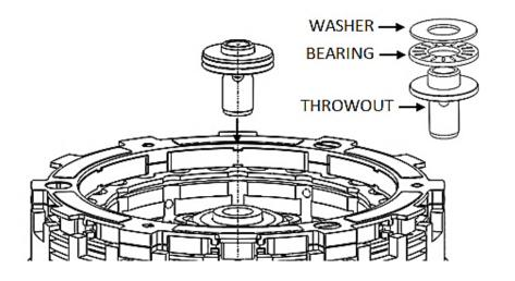
**NOTE:** If you are missing the top washer, it is probably stuck to the backside of your OE pressure plate.
