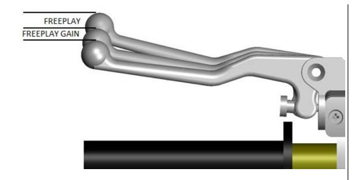
Optimal Freeplay Gain yields ~1/8" (3mm) of clutch lever movement, measured at the ball end of the lever. measurement This at the lever correlates to achieving the ideal installed gap, so you will use the Freeplay Gain measurement to accurately set the installed gap.
