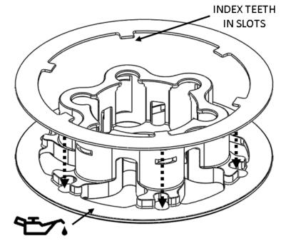
**11.** Install this pressure plate subassembly.
