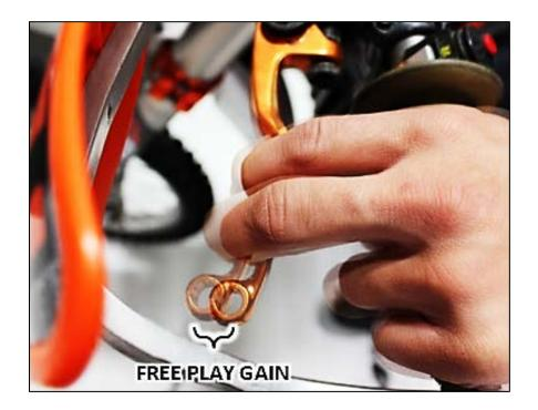
The following steps explain two ways to check Freeplay Gain. One will use the rubber band that has been included in the clutch kit and the other explains using your hand, which you will perform *before every ride*. effectively check freeplay gain every time you ride.
