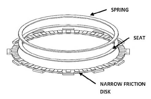
If judder spring and seat are installed, assemble the clutch in the following order.
